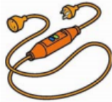
Figure 3 Portable safety switch fitted directly to power cable
