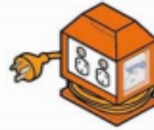
Figure 4 Portable safety switch protected power board
